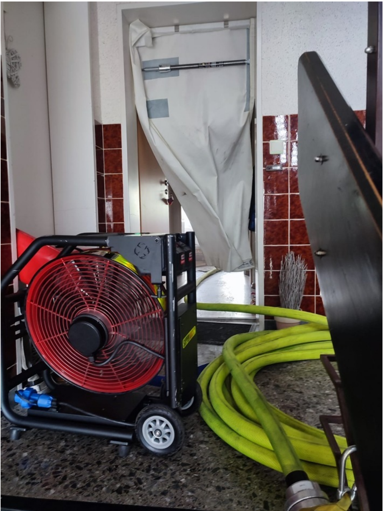
Smoke apron in the entrance area © Feuerwehr
