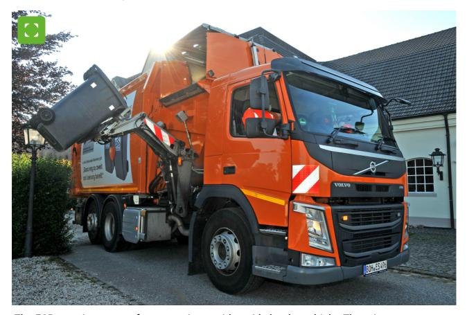
*The ESB empties most refuse containers with a side-loader vehicle. The gripper arm grasps a residual waste bin and empties it at the top of the loading opening. The driver in the picture is Maik van Drünen.* © Foto: Bruno Wansing, Stadt Bocholt
