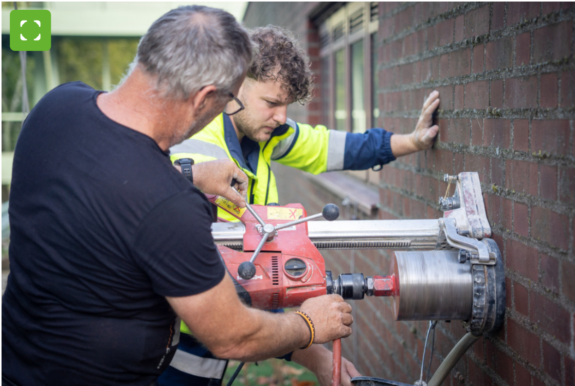
Building inspectors Michael Krings (left) and Anton Zimmermann from the Cologne-based company Finette + Schönborn take the wall sample.
